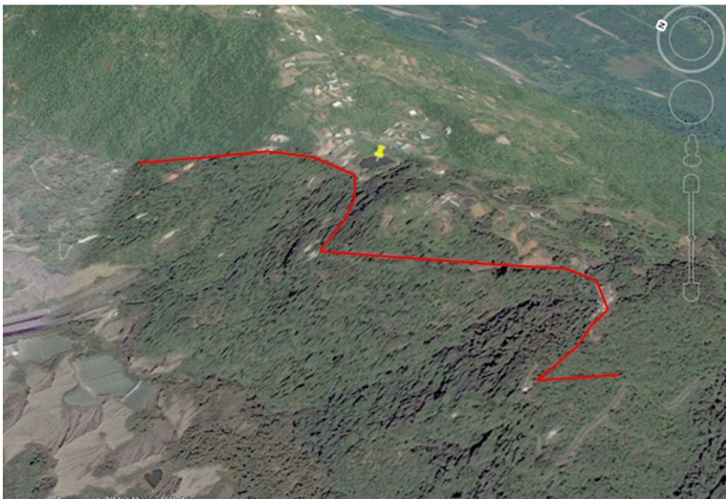
(c) \Omega -shaped bends typical of mountainous regions (Background image from Google Earth, 2019).
