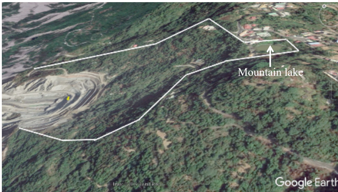
Figure 5. The area of influence of water from the mountain lake above the Zhongliao Tunnel (Background image from Google Earth, 2019).
